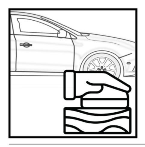
1. After a good preparation to the repair area, flat the whole panel with P1000-P1500 dry or P1500-P2000 wet to ensure good adhesion and to avoid dark arches.
