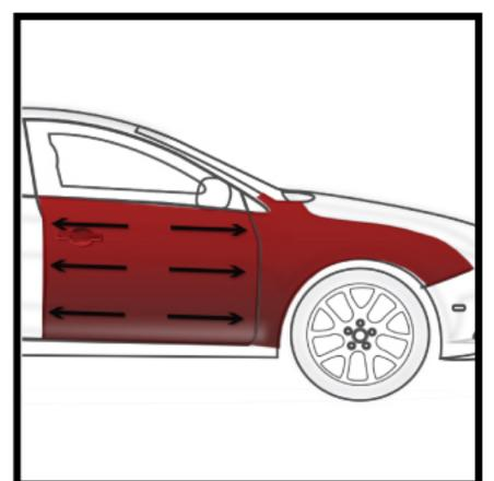
2. Apply the basecoat to the defined repair area as per technical data sheet.
