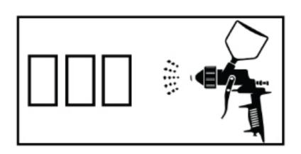
6. Apply 1 final UNTINTED 2K clearcoat to all panels, simultaneously, as this will have an effect on the final shade and result.
