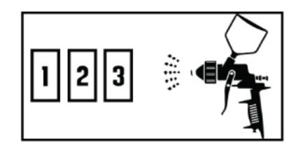
1. Apply the correct colored primer, as given by Genmix, to 3 test panels and flash-off or dry properly.
